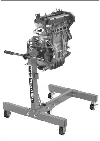
9. Once you are confident that the stand is supporting the weight of the engine, disconnect the hoist. Now that the engine is mounted to the stand it can be rotated around to access all sides of the engine. Use the locking pin to lock the engine at one of four different working angles.
